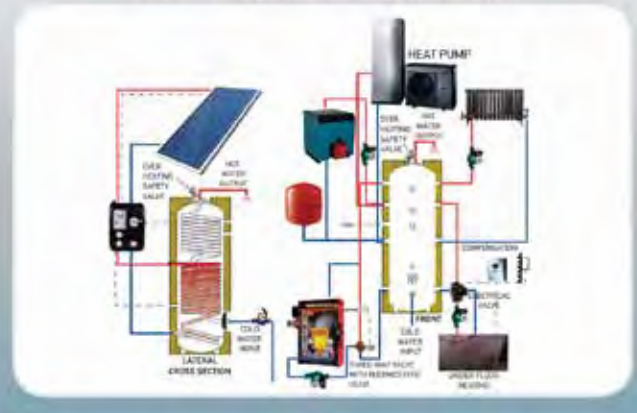
Typical Installation Buffer-1 Tank with INOX heat exchanger for Domestic Hot Water
